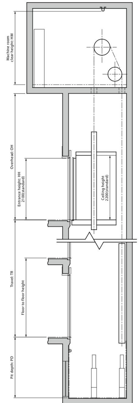
Note: Hoistway section for side-drop counterweight (1-door 1-gate & 2-gate) is slightly different from this figure.
